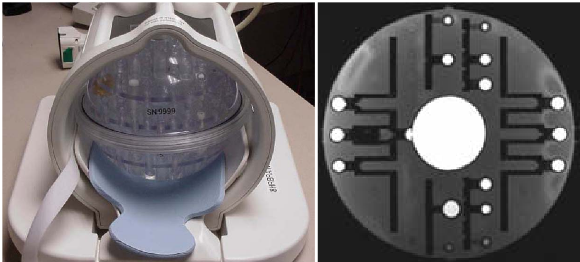
Figure 3. The image on the left shows the phantom placed in the correct position, with the Serial Number (SN 9999) facing out. This will be the typical scanning position for your phantom. The image on the right shows a typical sagittal MRI image of the phantom.
